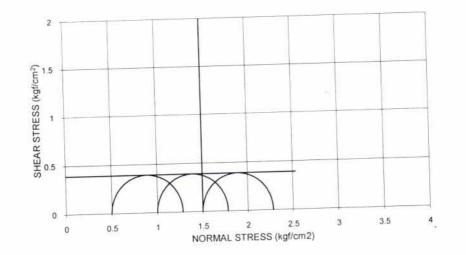
BH NO: 9 DEPTH: 3.5 m  $_{C} = 0.39 \text{ kgf/cm}^{2}$  $\Phi = 0.0^{\circ}$
